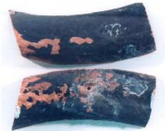
Pit in copper tubing
