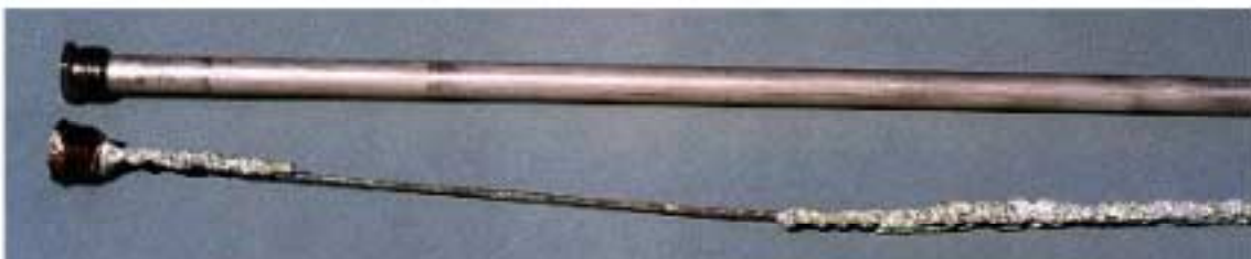
Comparison of a new anode and a spent anode
